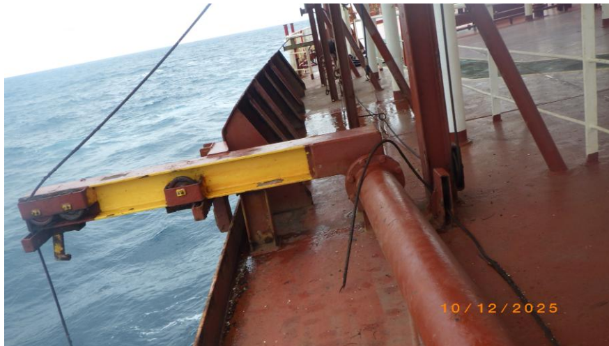
Figure 8b – Parted wire rope ( Source: the Company )
