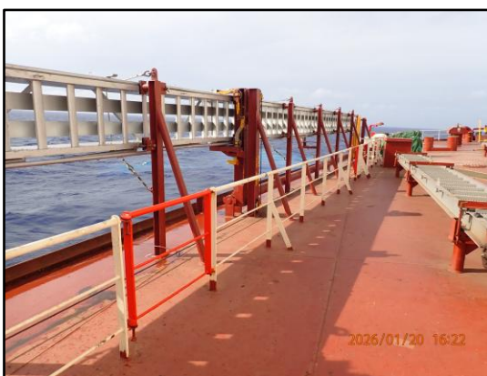
Figure 1 – View of the starboard gangway in secured position. (Source: the Company)
