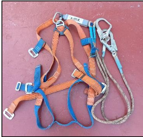
Figure 2 – Safety harness available onboard Legacy that the BSN used on the day of the occurrence. (Source: the Company)
