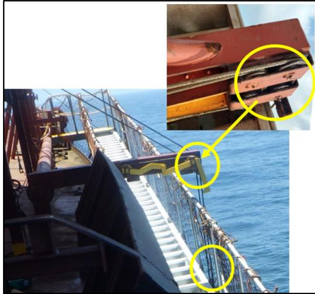
Figure 3 – View of upper and lower outer sheaves on starboard gangway for illustration.
